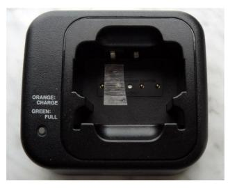
Build a jumper between the original Yaesu CA-9 base charging stand and connect to the terminals of BC119N using crocodile clips. See below:
